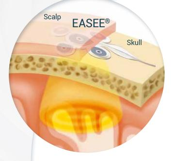
The special shape of the electrode ensures that the stimulation reaches the desired location in the brain from outside the skull.
